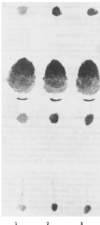
Figure 1 —Typical thin-layer chromatogram. Key: 1, salicylazosulfapyridine; 2, salicylazosulfapyridine tablets (recent lot); and 3, salicylazosulfapyridine (a lot several years older).
